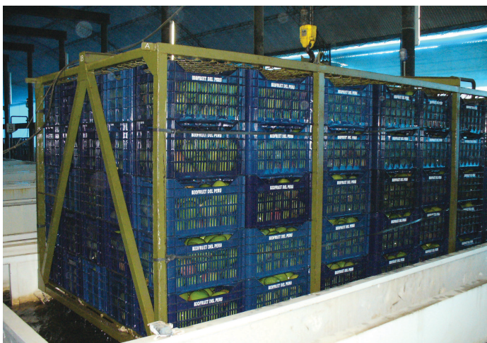
Mangos being lowered into a hydrocooler
