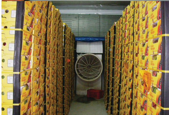
Forced-air cooling tunnels
