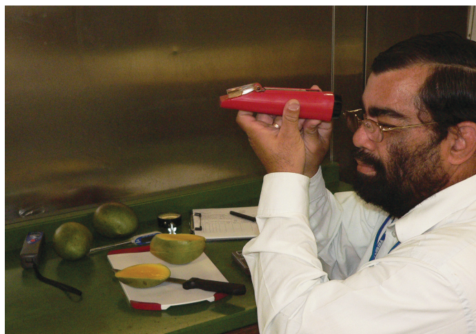
Measuring mango fruit TSS with a refractometer
