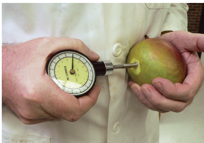
Measuring mango flesh firmness with a penetrometer
