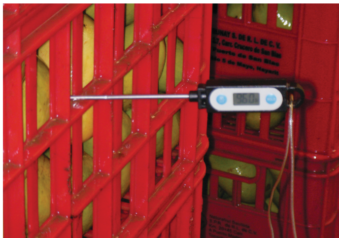
Measuring mango flesh temperature following hydrocooling
