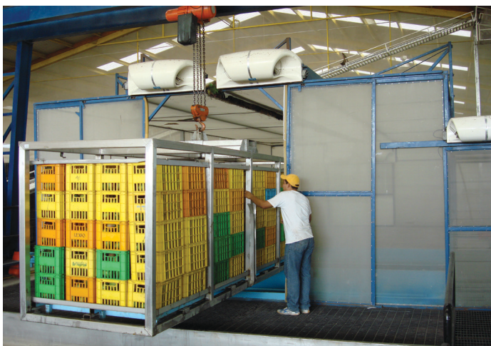
Post-hot-water treatment hydrocooling
