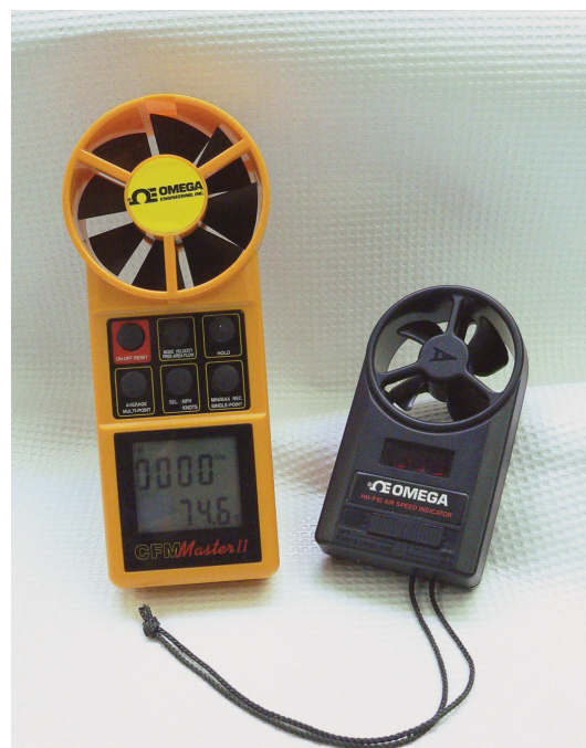
Vane anemometers used to measure air velocity
