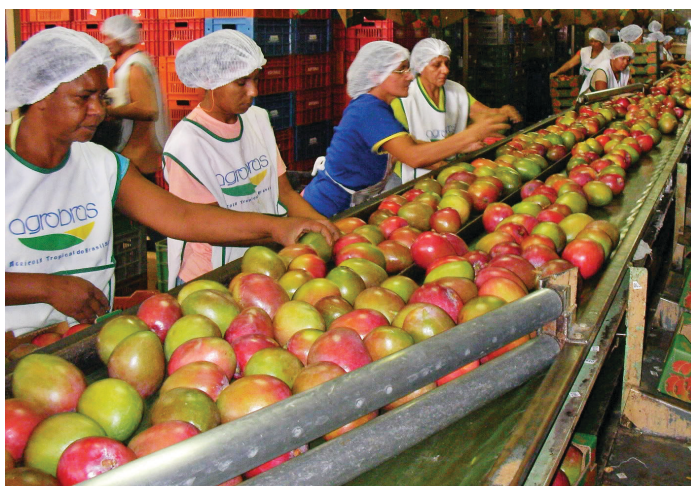
Manual fruit sizing and carton filling
