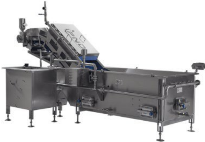
Figure 3. Prewash tank Credit Pnd Srl - PREP-WASH
