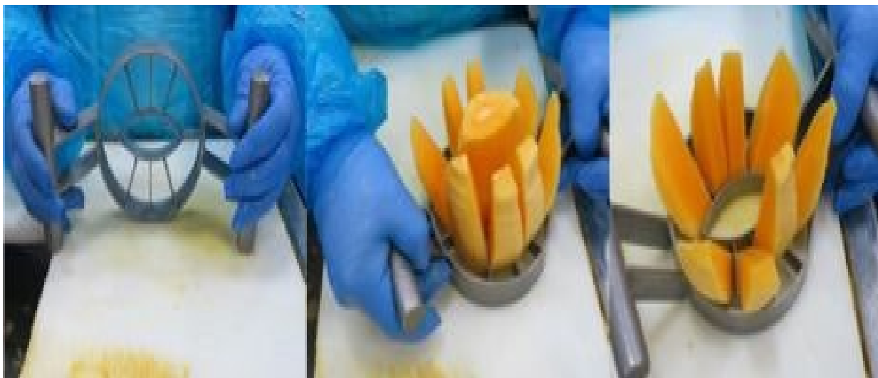
Figure 21. De-pitting and slicing of mangos by hand with a specialized instrument. Credit: Fresh Del Monte Produce, Inc.
