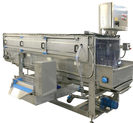
Figure 4. Prewash tank Credit SWC Industrial Fruit Washing Systems | ABL (ablcavezzo.com)
