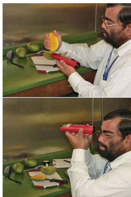
Figure 34. Measuring mango fruit SSC with a refractometer.
