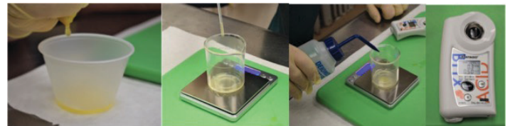
Figure 36. A pocket Brix-acidity meter. Note: Juice samples need to be diluted 1:50 to measure total acids. (Pocket Brix-Acidity Meter | ATAGO CO., LTD.) Credits: Sandra Matlack, USDA, ARS, Fort Pierce
