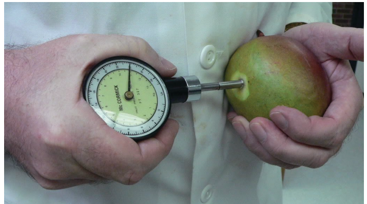
Figure 42. Measuring firmness with a handheld penetrometer.
