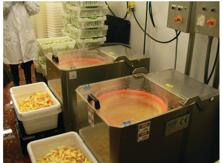
Figure 19. If fresh-cut mango slices are treated with a liquid supplemental treatment, they may be centrifuged to remove the excess liquid, as shown here for apple slices, following immersion in calcium ascorbate solution.
