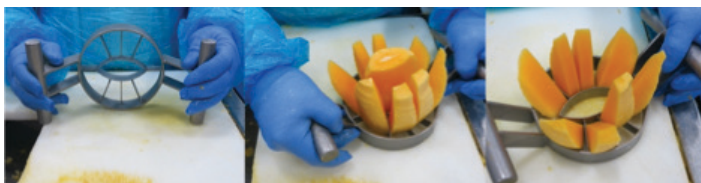
Figure 16. De-pitting and slicing of mangos by hand with a specialized instrument. Credits: Fresh Del Monte Produce, Inc.
