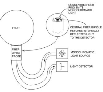
chemical composition of the flesh just below the skin be well correlated to the chemical composition of the whole fruit. Figure 1. Interactance probe used to make nondestructive optical absorbance measurements of fruit.
