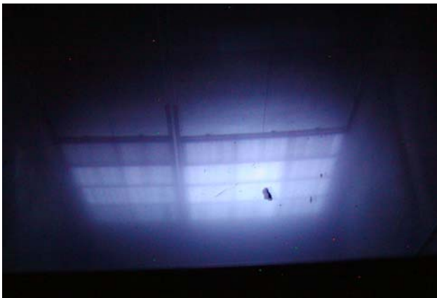
Cobalt 60 radiation source under water when product is not being treated
