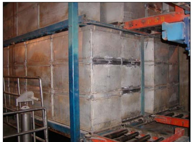
Position of totes when product is being exposed to radiation source
