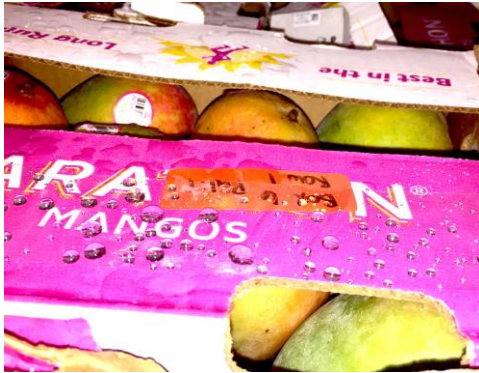
Figure 11: Condensation on Mangos and Cases with the Metalized Bubble Wrap Cover with Base
