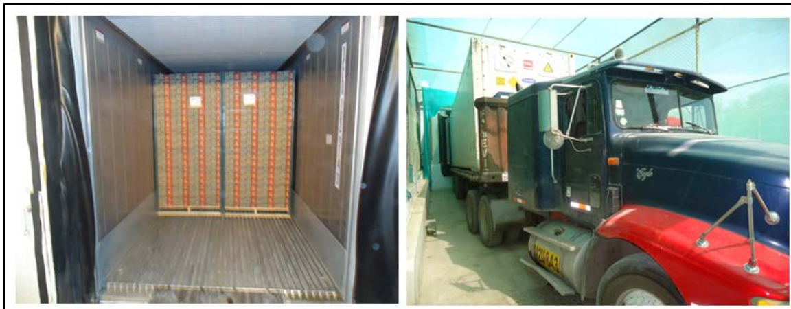
Figure 7: Palletized Loads Inside Pre-Cooled ISO Intermodal Container
