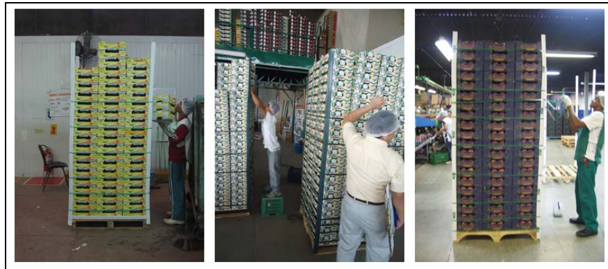
Figure 6: Palletizing of Trays and Use of Plastic Bands to Secure Loaded Pallets
