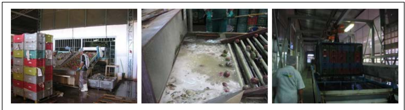
Figure 2: Incoming Fresh Mangos Received in Plastic Totes, Washed and Hydro-Cooled
