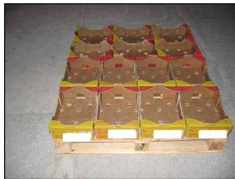
Figure 10: 14 down Foot Print on a Non-GMA Pallet
